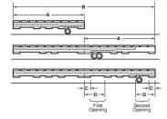
pallet. On models with a single load wheel, the "C" dimension should be 6" maximum and the "D" dimension should be 14" minimum. On models with tandem load wheels, the "C" dimension should be 6" maximum and the "D" dimension should be 17" minimum. Customers that need tandem load wheel trucks, but use pallets with smaller openings, may be accommodated if the maximum lift height of the truck is reduced. Contact your Crown dealer for details
