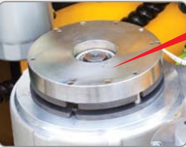
Electromagnetic brake controller parameters is mounted on the traction motor.
